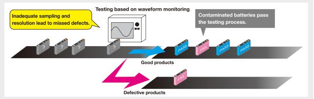
In order to detect contamination, it's common to check voltage and current waveforms applied by a waveform measuring instrument. However, contamination may not be detected depending on the instrument's waveform detection capability, contaminated batteries may be released to the market.
