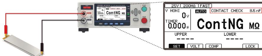
This issue can be resolved with the BT5525's contact check function. The function measures the capacitance between measurement terminals (including stray capacitance and the capacitance of the circuit under test) to generate a pass/fail judgment. The capacitance values measured by the contact check function can be used to manage contact status in a quantitative manner.
